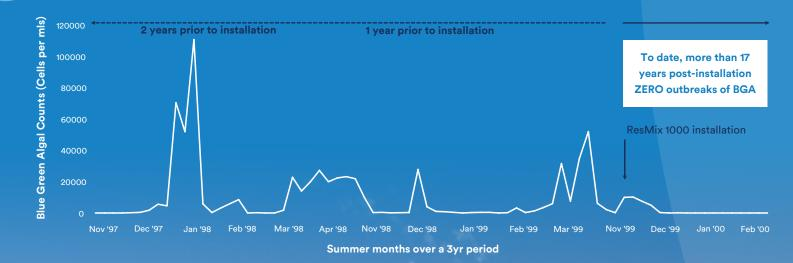
Data captured over the summer months pre- and post-installation of the ResMix system show outbreaks of Blue Green Algae (BGA) in the water reservoir in the years prior to installation. The ResMix system, installed in 1999 has resulted in zero occurrences of BGA in this reservoir since – more than 17 years.
