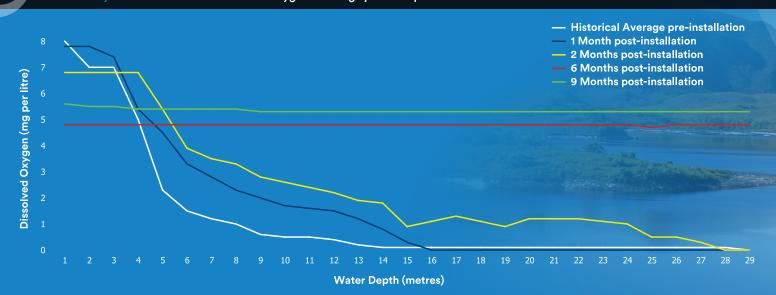
Following installation of the ResMix system, results show that the water is immediately impacted by the ResMix system and within 6 months, is uniform and continues to increase in oxygenated water to a consistent and uniform 6mg/L from top to bottom of the water reservoir 9 months after installation.
